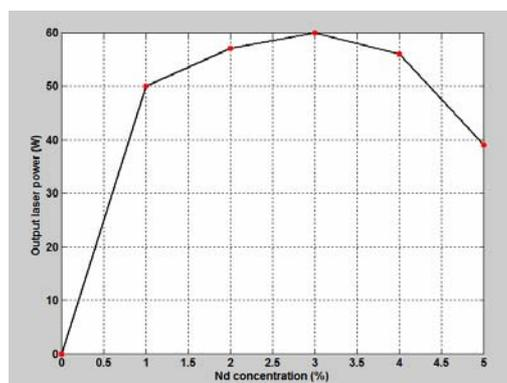
**Figure 6.** Dependence of output laser power on neodymium concentration for ceramic Nd:Ce:YAG disc laser
