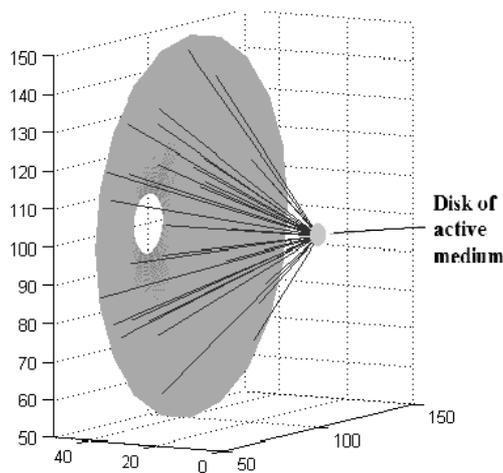
**Figure 1.** Scheme of a disc laser pumped by parabolic solar concentrator
