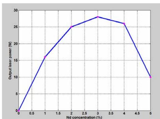
**Figure 5.** Dependence of output laser power on neodymium concentration for ceramic Nd:YAG disc laser
