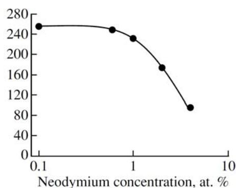
**Figure 4.** Dependence of upper laser level lifetime (in microseconds) on the neodymium concentration [4]
