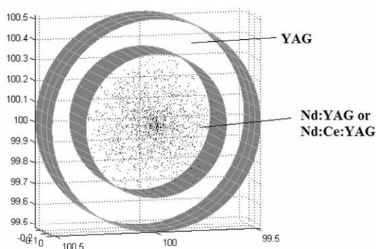
**Figure 3.** Core doped disc type active medium with distribution of absorbed photons
